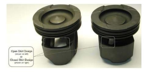
Care must be taken when replacing less than full sets of pistons within an
