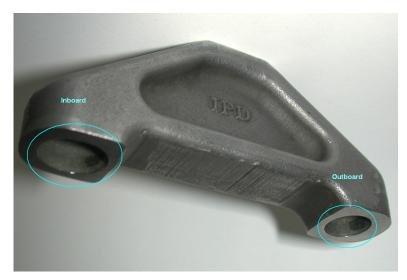
An imbalance of the valve bridge can be caused by mismatching the valve springs. The same springs must be used on both valves under the common bridge. If a lower load spring is used on either valve under the same floating bridge the bridge will be imbalanced. At a minimum an imbalance can accelerate valve guide and valve stem wear. If the imbalance is severe, it can exert enough force to fracture the valve stem at the keeper grooves.
