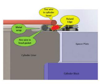
Finally, an additional option used alone or with either of the previous ideas is using one of the composite metal repair compounds to fill the cutouts (voids) in the head.
