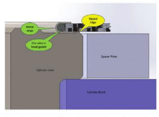
layers of metal core, so there has to be enough room between the wire and raised edge for the gasket layers to form between.
