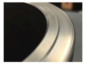
The concept is to create a raised ridge on the top of the liner flange that bites into the head gasket.
