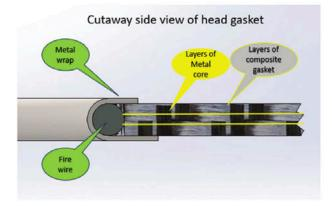
The composite gasket is cut so the firewire sits just inside it. Over time as the gasket migrates into the cutout voids between the cylinders, it pulls away from supporting the back of the firewire and structurally weakens the gasket.
