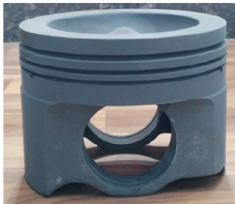
Shown above, prior to deburring (left) and after deburring (right). Shown below, a piston after phosphate coating and screen printing.
