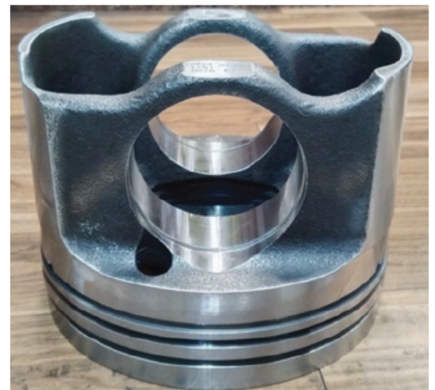
Shown above, prior to deburring (left) and after deburring (right). Shown below, a piston after phosphate coating and screen printing.
