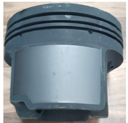
Shown above, prior to deburring (left) and after deburring (right). Shown below, a piston after phosphate coating and screen printing.
