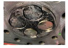
there was less than 40 miles on the engine, the question remains whether the piston or liner was defective or out of specifications?
