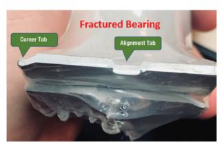
A fractured connecting rod has a 0.032" larger bore for the rod bearing than a saw-cut rod.
