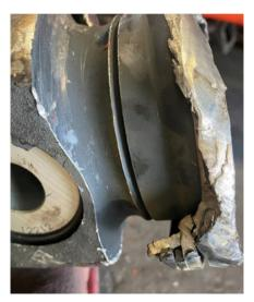
There was a piece of the APR ring jammed into the head. Did the APR ring fail? If you skip ahead to the conclusion of this article you forfeit any remaining kudos.
