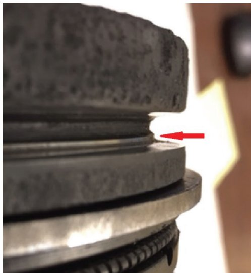
The ring land of this piston has worn leaving a ledge at the back on the ring groove.
