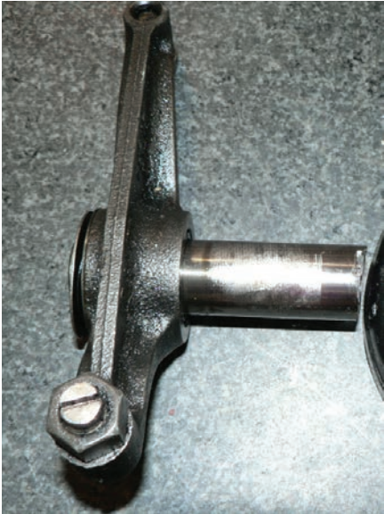
Closer inspection of the bracket found the alignment dowel in this bracket has been severely damaged.
