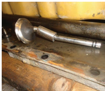
The other valve from the failed cylinder is bent and the guide is broken.
