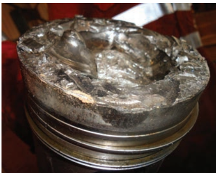
The head of the valve is lodged in the crown of the piston. There're no signs of piston seizure.
