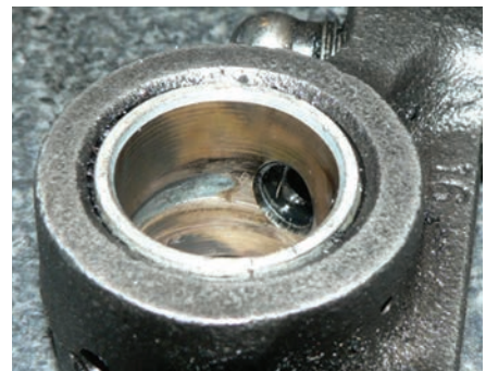
The rocker arm closest to the fracture of the shaft had evidence of uneven wear and scoring. This rocker arm is positioned directly over the fracture in the rocker arm shaft.
