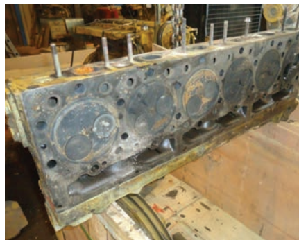
The cylinder head is damaged, and the valves are no longer in the failed cylinder.
