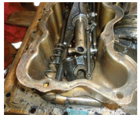
Assorted rocker arm components and push rods were removed and stacked in the valve cover.
