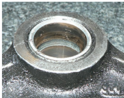
The rocker arm closest to the fracture of the shaft had evidence of uneven wear and scoring. This rocker arm is positioned directly over the fracture in the rocker arm shaft.
