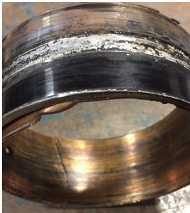
Failed Cam Bearing From Dry Start-Up
