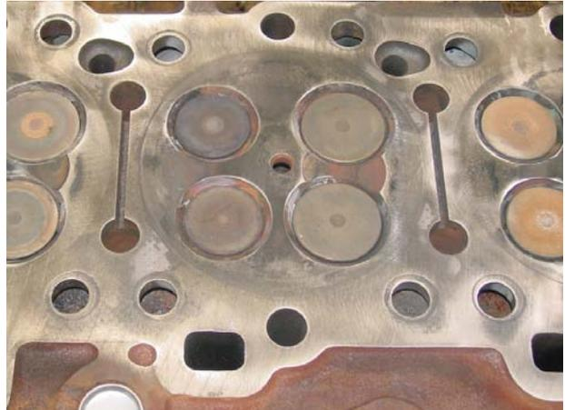
As the C15 engines gained in popularity, the OEM began using these “relief cut” heads in their exchange program for both 3406E & C15 engines. This presented a problem for engine owners that had the older style blocks.
