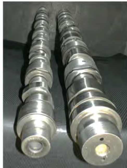
The injector camshaft is massive in comparison to the valve camshaft, with a journal diameter of approximately 85.0 mm (3.346") compared to the journal diameter of approximately 65.0 mm (2.559") of the valve cam.
