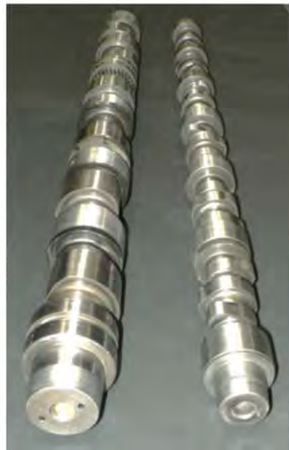
The injector camshaft is massive in comparison to the valve camshaft, with a journal diameter of approximately 85.0 mm (3.346") compared to the journal diameter of approximately 65.0 mm (2.559") of the valve cam.
