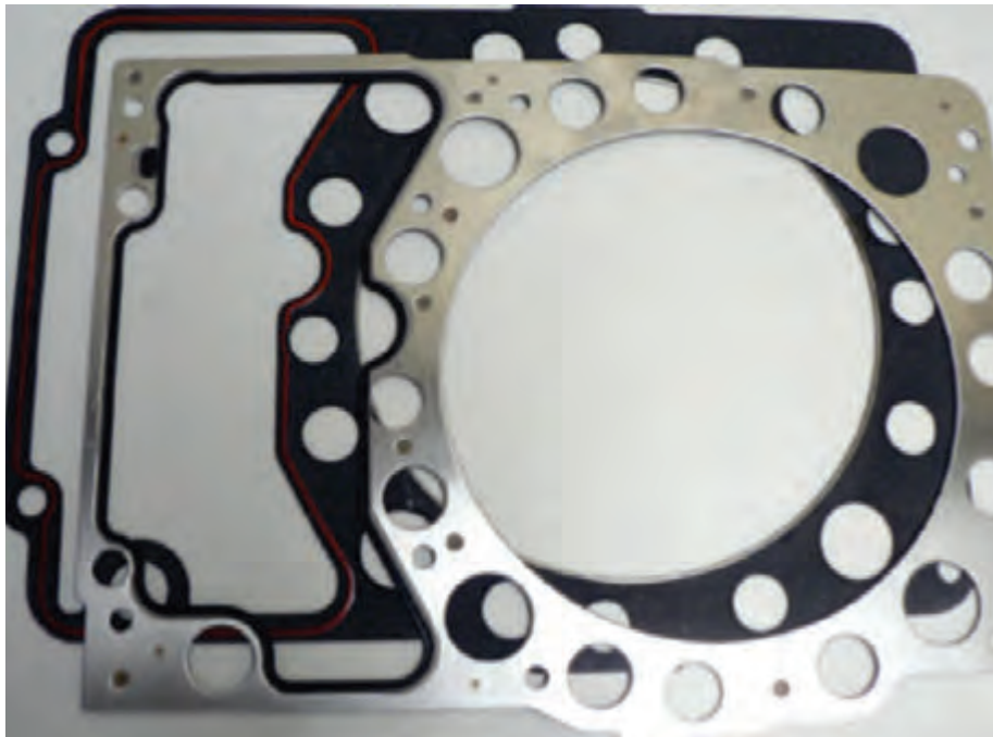
A Multiple Layer Steel (MLS) Head Gasket is pictured top and a Composite Head Gasket is shown beneath it.
