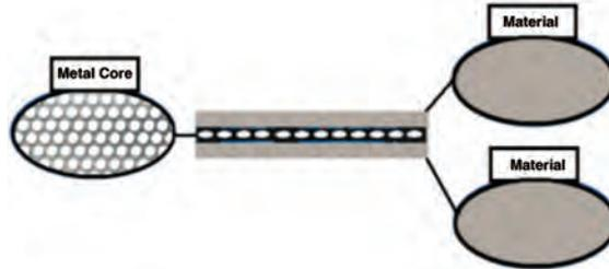
**Figure 3.** Later Style Head Gasket
