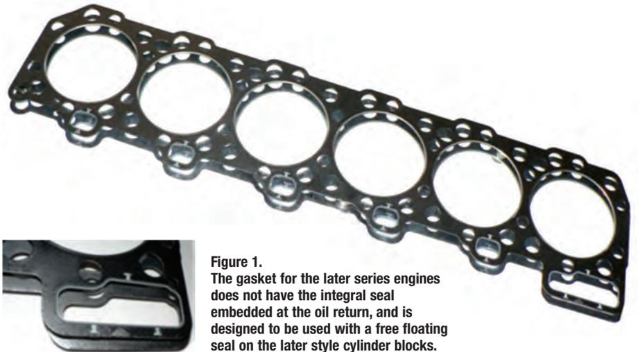
**Figure 1.** The gasket for the later series engines does not have the integral seal embedded at the oil return, and is designed to be used with a free floating seal on the later style cylinder blocks.
