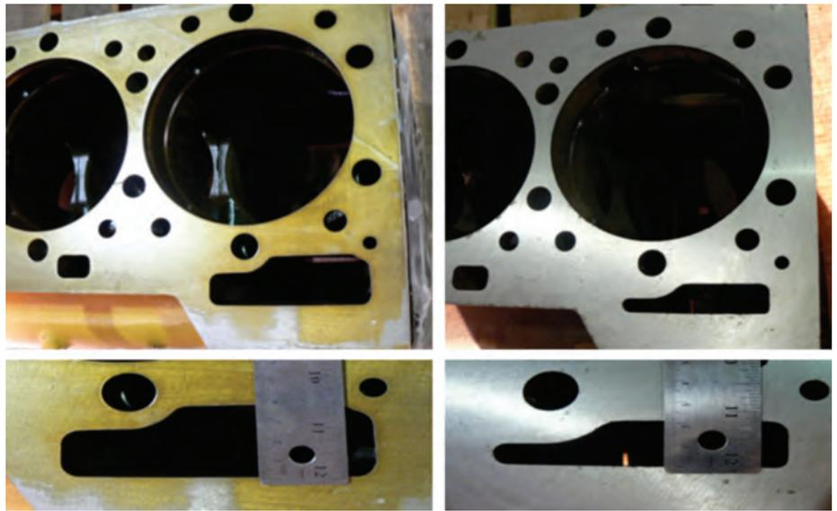
Figure 5. Block deck differences, prior on left; current on right.
