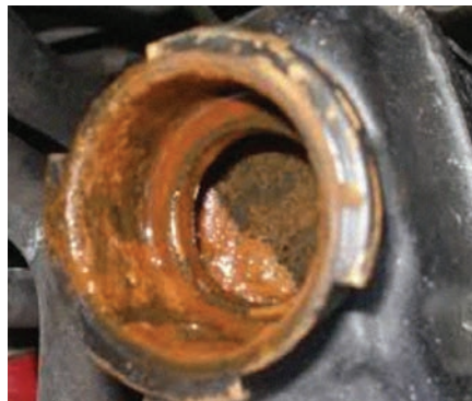
Rust and corrosion in the radiator.
