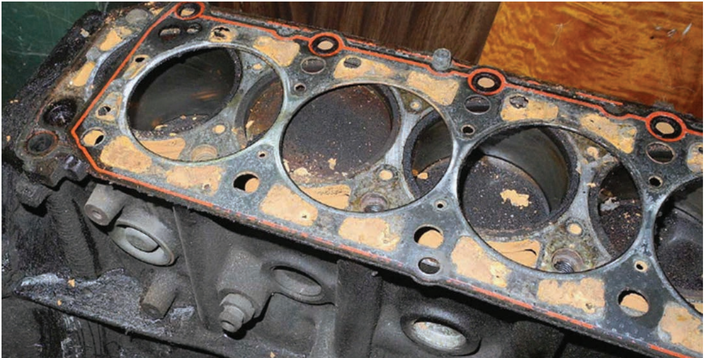
Rust already in the coolant passages.
